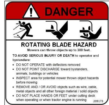
209173 ROTATING BLADE HAZARD
