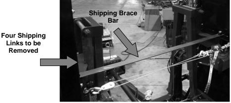
3) Tighten the device until enough tension is relieved from the shipping brace bar. Remove the wire securing the flat bar to the wing, and the flat bar itself.
