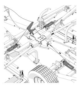
Operators must check the operation of the Pro Lift-N-Turn™ system prior to the start of each shift. Ensure that each latch plate is in the fully lowered (flat) position before starting to mow.
