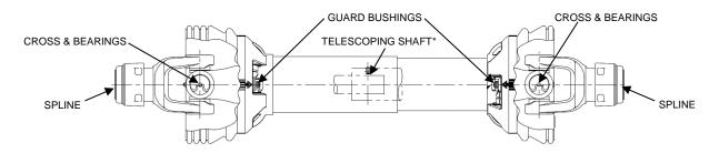
\* Inner & outer guards must be rotated to align holes for accessing telescoping shaft grease fitting.
