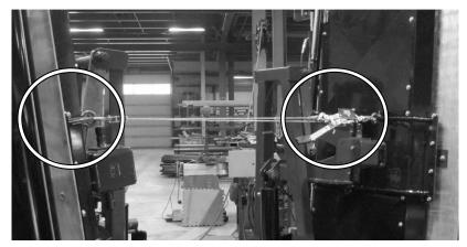
2) With the TDR Spreader Fixture (526498) in place, attach a ratchet equipped strap between both wing decks using the points shown.
