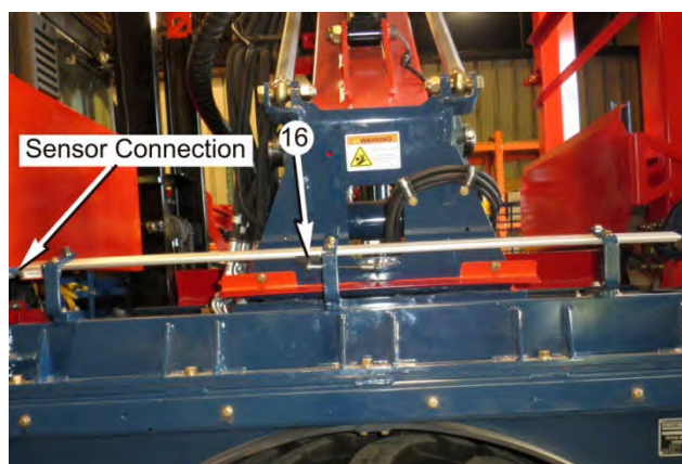
16. Arm Rail Sensor.No adjustment.
