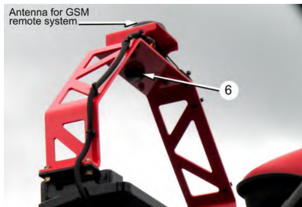
6. Mast 'Height' Sensor. No adjustment. Part No. B500210 – Ultrasonic Sensor w/Decal
